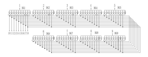
"△" represents Internal Circuit Feature: A、C、E…Common Cathode, B、D、F…Common Anode.
