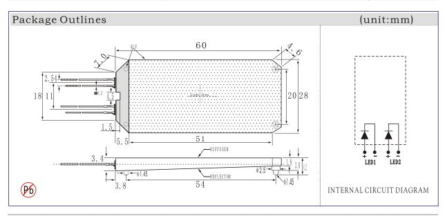
Remark: 1. "\(\triangle^{"}\) represents Internal Circuit Feature: A, C, E...Common Cathode, B, D, F...Common Anode.
