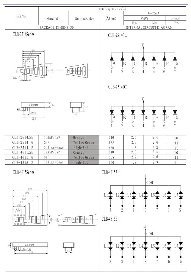
Remark : 1. "△" represents Internal Circuit Feature: A, C, E…Common Cathode, B, D, F…Common Anode.
