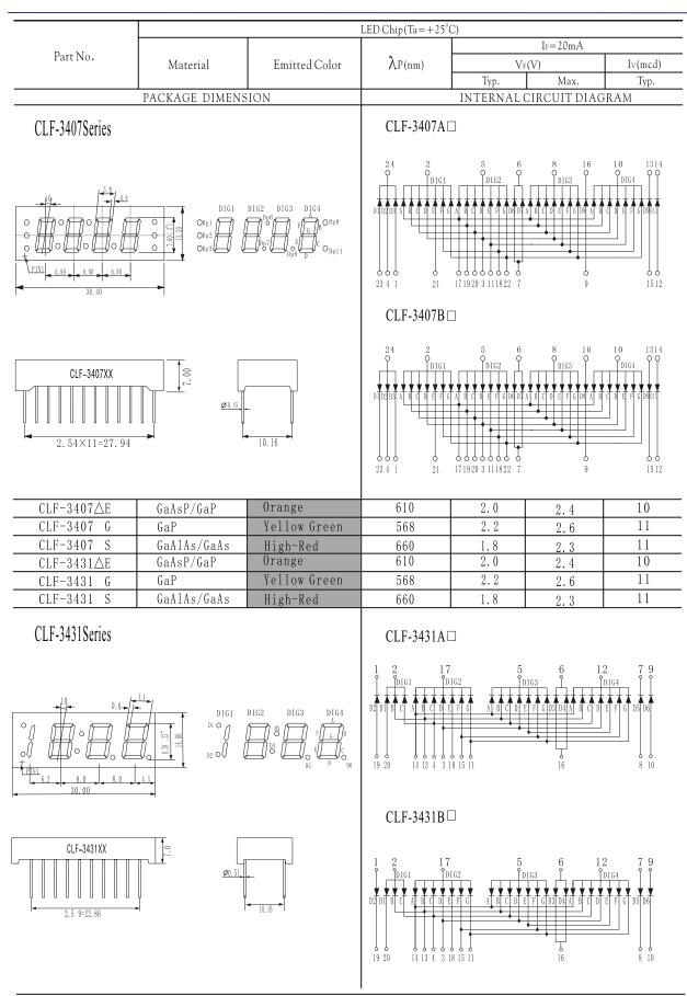
"A" represents Internal Circuit Feature: A, C, E...Common Cathode, B, D, F...Common Anode.
