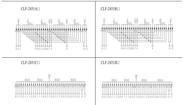
"△" represents Internal Circuit Feature: A、C、E···Common Cathode, B、D、F···Common Anode.
